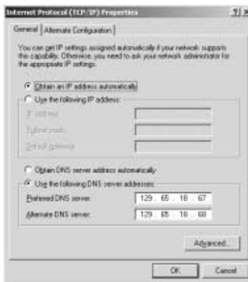
Using DHCP, normally no entries would be seen here (DHCP sets IP, DNS and all other TCP/IP settings). For this configuration we have forced DNS entries. As the campus moves to DHCP items in this dialog box will be left blank and all settings will be obtained automatically from the DHCP servers on campus.
