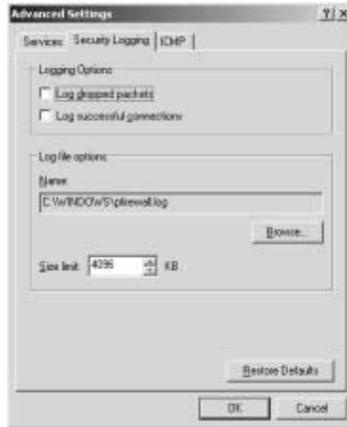
The personal firewall allows for you to maintain logs on important information (dropped packets, successful connections) and gives you the ability to set size limits.
